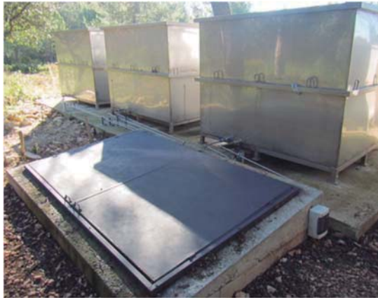
Fig. 2. Three lysimeters and their percolate collecting system
