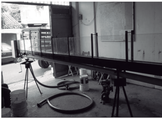
Fig. 2 Hydraulic jack, tripods and energy dissipation tank
