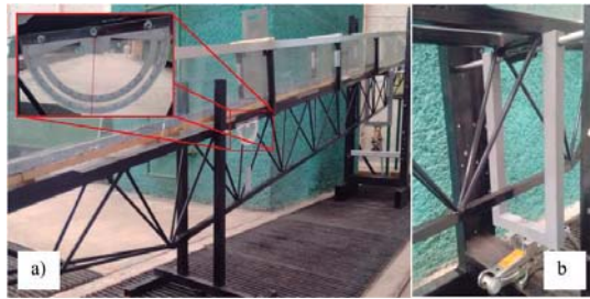
Fig. 1 Tilting flume (a) and lifting mechanism (b)
