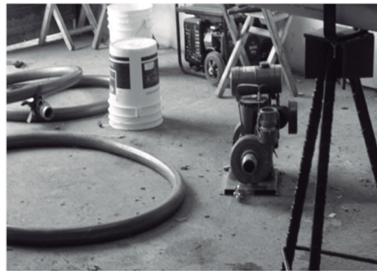
Fig. 4 4 HP gasoline pump
